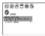
3. Press  $\blacktriangleright$  to lock ("X") or press  $\blacktriangleleft$  to unlock (" $\checkmark$ ").
